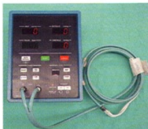
Dinamap blood pressure monitor. This is an oscillometric system. The display gives diastolic, systolic, and mean pressures and heart rate.
