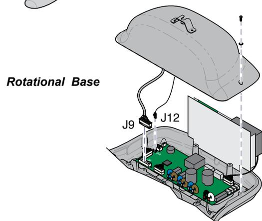
**Step 5: Disconnect foot actuator wires.**
