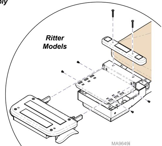
**Step 8: Remove jam nuts / pivot screws.**
