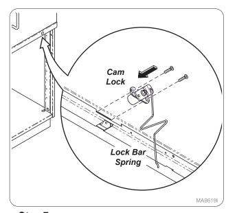
**Step 7:**Install cam lock inside cabinet with lock bar spring attached.
