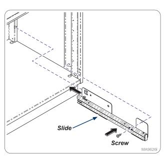
Step 12: Re-install slides (4) with screws (4).
