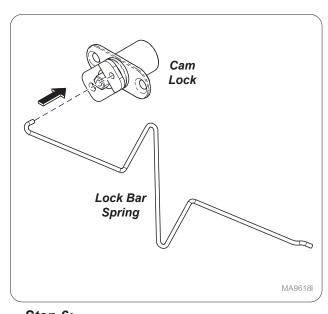
**Step 6:**Assemble lock bar spring onto cam lock.
