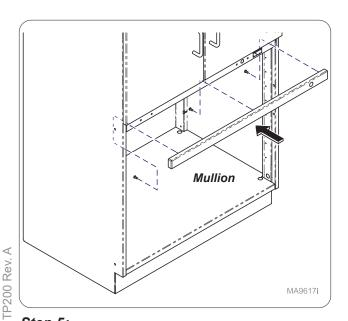
**Step 5:**Install mullion onto cabinet with screws(3).
