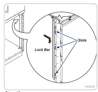
Step 10: Inside cabinet install lock bar into slots as shown. Note: Lock bars will vary but assembly process is the same.
