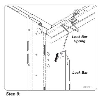
Install lock bar onto lock bar spring.
