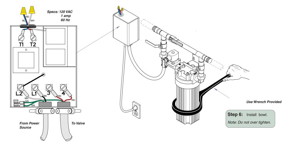
Step 7: Plug relay control box to 120 volt power source to energize electrical solenoid.
