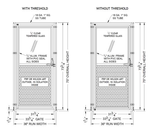
\*Gates are measured by Run Width and are available in one-inch increments from 29 to 42 inches wide.
