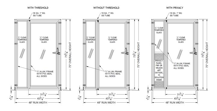
\*Stall Fronts are measured by Run Width and are available in one-inch increments from 43 to 72 inches wide.
