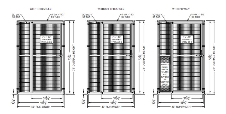
\*Stall Fronts are measured by Run Width and are available in one-inch increments from 43 to 72 inches wide.
