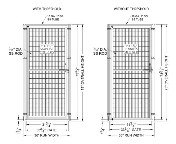
\*Gates are measured by Run Width and are available in one-inch increments from 29 to 42 inches wide.
