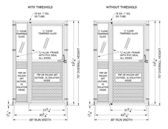
\*Stall Fronts are measured by Run Width and are available in one-inch increments from 43 to 72 inches wide.
