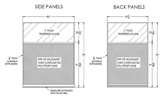
\*Side and Back Panel transfer doors cannot be combined in the same run
