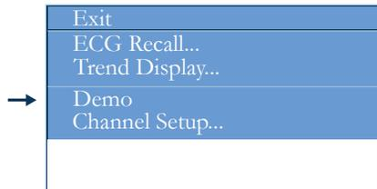
3. Press the Knob to display the Demo Mode Password Menu. Rotate the Knob to highlight the password box, and then press the knob to edit this field. A keypad will appear for your use. Rotate and press the knob alternately to enter the password: **8727**. Press the knob to confirm and exit that field.
