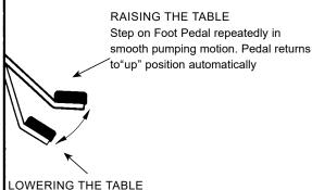
Depress Foot Pedal to bottom position to lower the table
