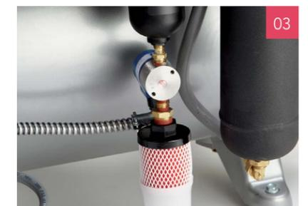
**03** Keep noise levels low with the exhaust silencer/filter.
