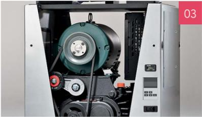
**03** The powerful 3-hp motor can meet the vacuum demands of up to 10 users simultaneously.
