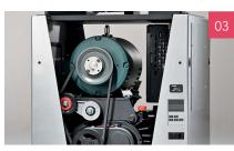
**03** The powerful 3-hp motor can meet the vacuum demands of up to 10 users simultaneously.
