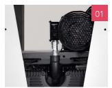
01 The PowerVac pump has an integrated silencer to reduce the noise level, making it one of the quietest dry vacuums on the market.
