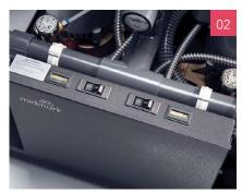
02 Separate twin model on/off switches and hour meters provide operational versatility.
