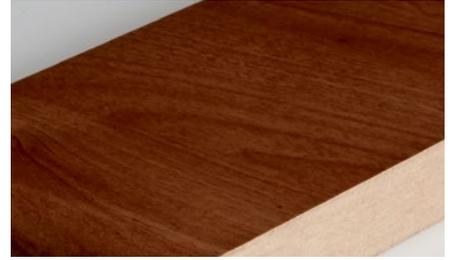
**Door and drawer core:** 45-lb LEED® IEQ-compliant MDF board, 3/4" thick (all composite wood material to meet CARB P2 emission standard of CARB regulation 91320.4)
