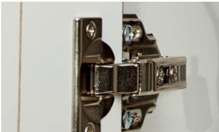
**Hinges:** Manufacturer's standard Blum® hinges; concealed, soft-close, 110° opening, nickel-plated metal, clip-on mount, three adjustment points
