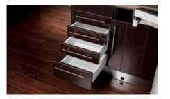
Drawer Systems: Soft-close, full extension Blum® TANDEMBOX™ intivo™ drawers (Silk White); full extension steel ball bearing slides, 100 lb capacity; 5/8″ THK 42-46# mediumdensity particle board core with thermally fused melamine coating (white) bottom and back
