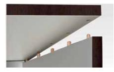
**Structure:** 3/4" THK 42-46# medium density particle board core with thermally fused melamine coating (white); glued wood dowel frameless construction
