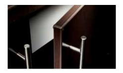
**Door and Drawer Fronts:** 3/4" THK 42-46# medium-density particle board core with thermally fused melamine coating (standard color offering) with 3-mm PVC edgebanding
