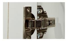
**Hinges:** Manufacturer's standard Blum<sup>®</sup> hinges; concealed, soft-close, 110° opening, nickel-plated metal, clip-on mount, three adjustment points
