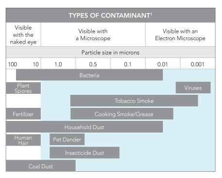
Contaminants that pass through a 5-micron filter
