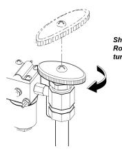
Shut-off Valves Rotate clockwise 1/4 turn to Shut off.
