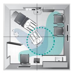
Barrier-Free Access: The center of the room is kept open to allow a 60-in wheelchair turning area and the transfer of the patient onto the exam chair. The distance from the door to the corner of the room (18 in) is needed for patient egress.
