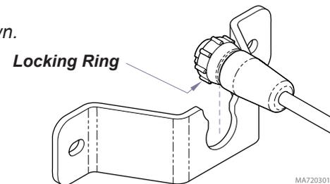
**Step 4:** Connect hand/foot control to cord inlet. Tighten locking ring.
