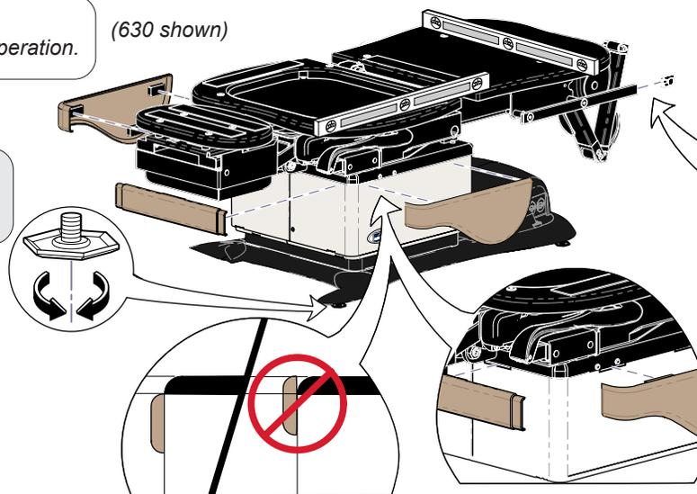
**Step 7:** Install hand control mounting discs (2), and holster.
