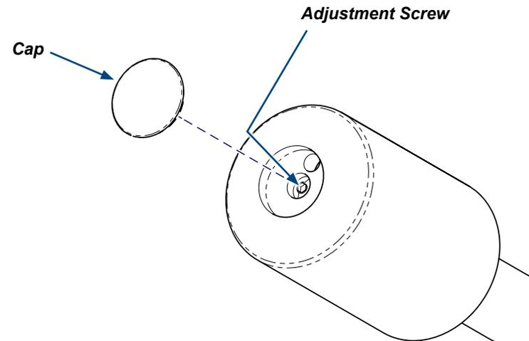
**Step 19: Adjust ball pivot tension...**
