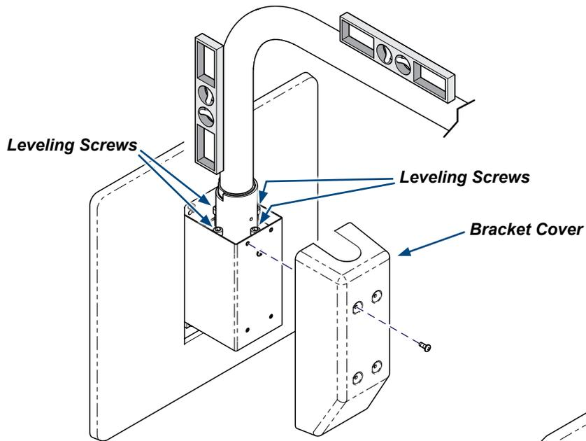
**Step 15: Level fixed arm / install bracket cover.**
