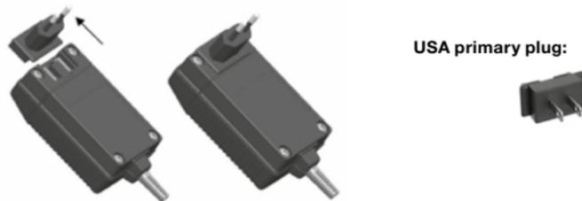
The mains socket adapter of the power supply is interchangeable, this enables worldwide operation. The pictograms describe the procedure of changing the adapters.
